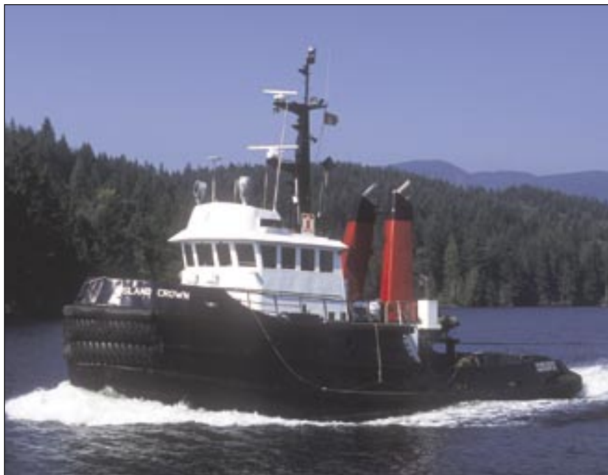
Island Tug & Barge's Island Crown has been re-engined with new Cummins KTA 38s rated at 500 hp at 1,600 rpm and 900hp at 1,800 rpm. Photo by kevinmillerphoto.com, courtesy of Island Tug & Barge.
